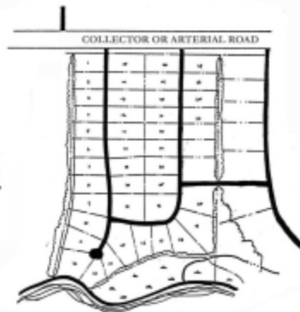
PARALLEL PLAN - ILLUSTRATES APPROXIMATE LAYOUT OF STREETS, BLOCKS AND LOTS BASED ON CONVENTIONAL STANDARDS (SEE SECTION 3.5, SUB-SECTION 2)
